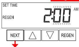
**Step 5I** – Next Regeneration Time (minutes): Set the minutes of day for regeneration using ▲ or ▼. This display will not be shown if “on 0” is selected in Set Regeneration Time Option in OEM Softener System Setup or OEM Filter System Setup.
