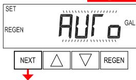
**Step 11S** – Set Volume Capacity using ▲ or ▼. If value is set to:
